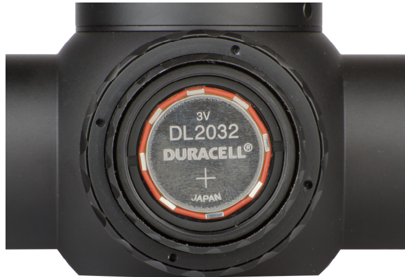
Fig. 2n View of battery cap removed. Note battery is positioned with positive (+) side out.
