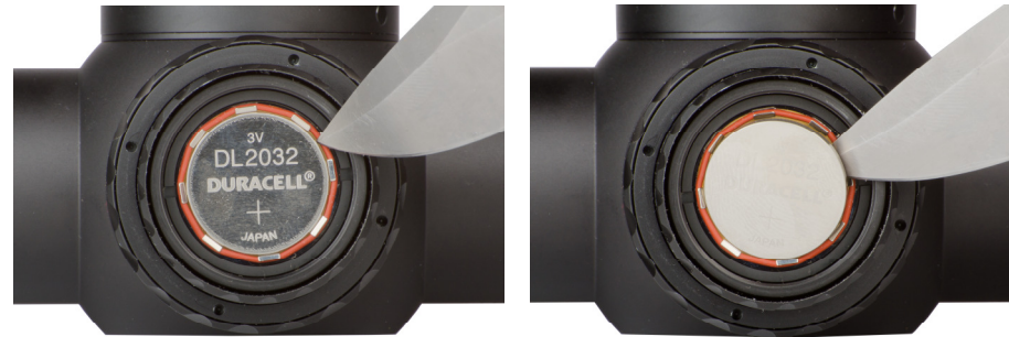
Fig. 2o Place the tip of a pointed tool between the battery edge and the orange tensioning ring to gently pry the battery out. Be careful not to cut the tensioning ring.
