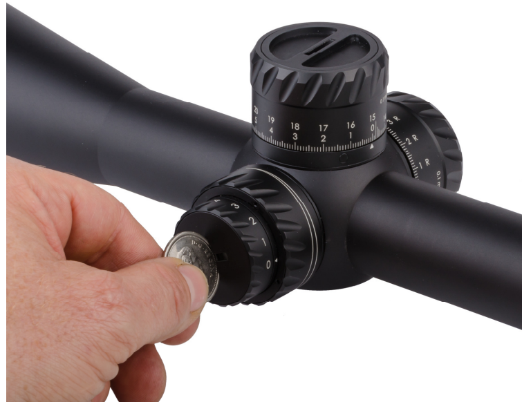
Fig. 2m Removing and installing the battery cap with the use of a coin. To avoid damage, use the slot that best fits the thickness of the coin.
