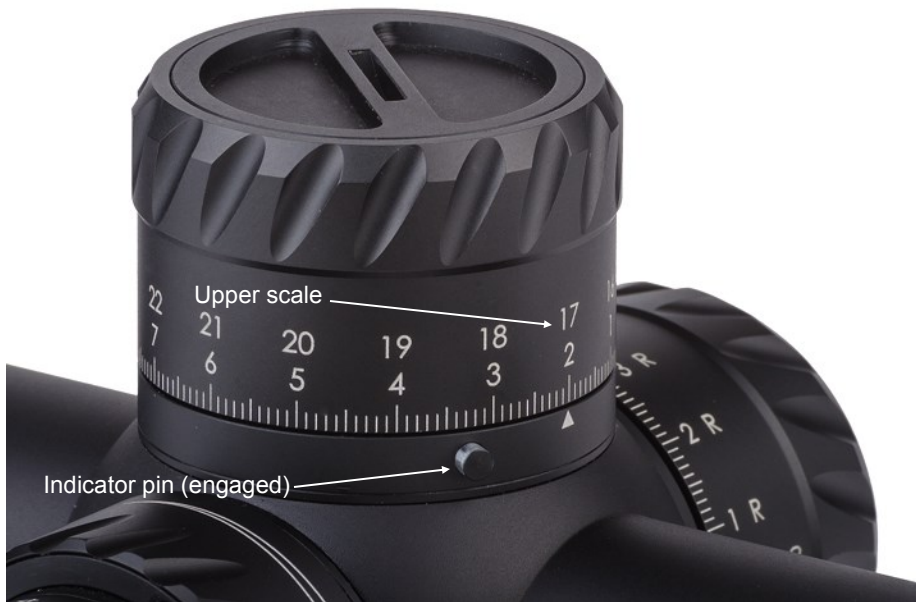
Fig. 2i Elevation Dial on second revolution. Read graduations from upper scale. Note indicator pin is engaged.
